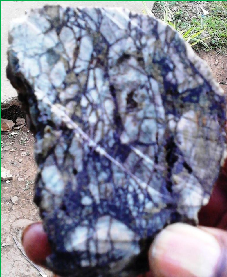
Crackle Breccia-later filled and cut by magnetite-pyrite-chalcopyrite
